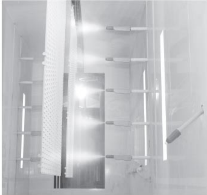
Above: An interior view of the powder booth's automatic guns during a coating process.
