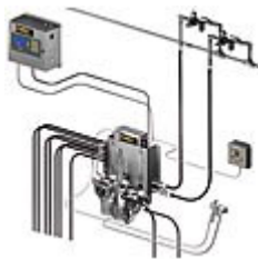
Figure 1. A typical electronic proportioning system includes two key pieces of hardware: the controller (above left) and the fluid panel (center).
